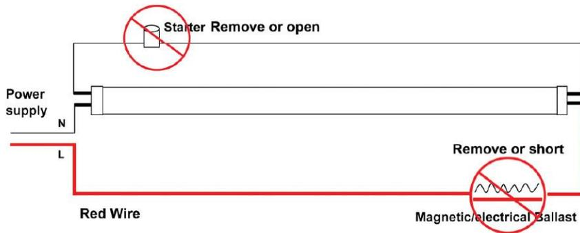
Wiring Diagram for LED Retrofit to Fixture with Magnetic Ballast
